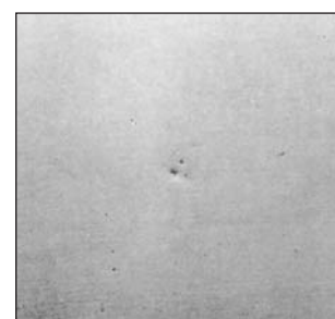
Pinhole texture by inappropriate rust proof.
