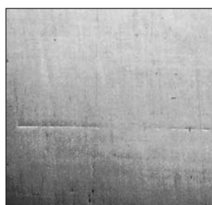
Scratch remains due to overload.
