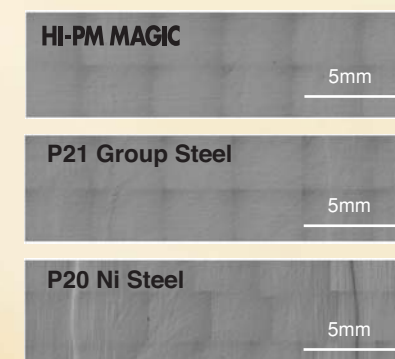
Differential interference micrographs comparison of the polish surface after welding
